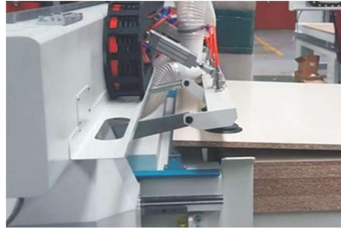
Automatic feeding of planks
