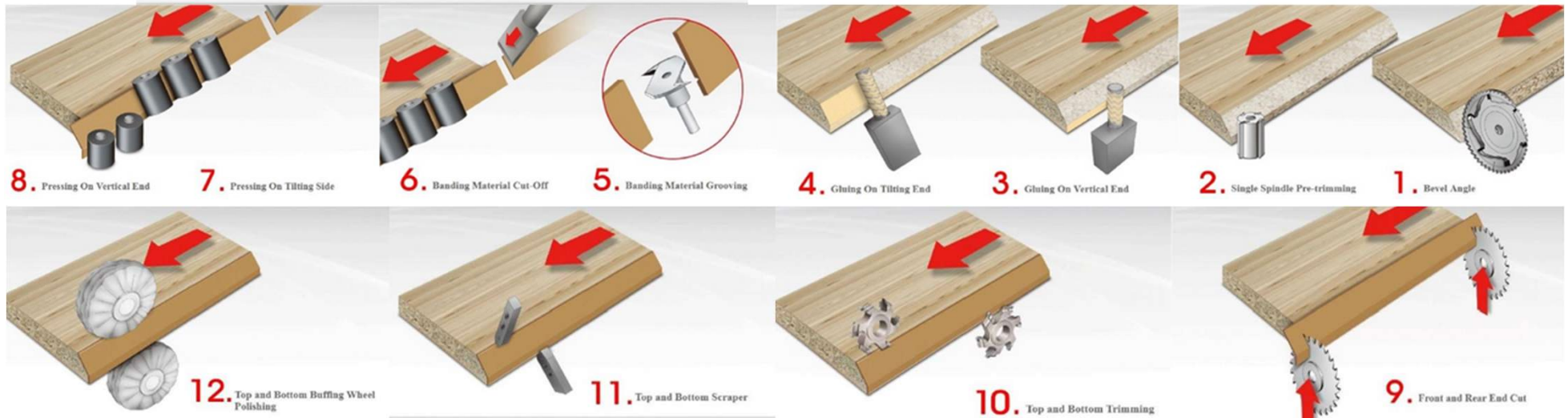
Inclined Side Processing Flow Chart
