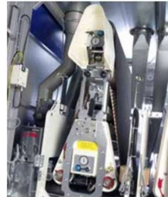
Longitudinal sanding unit (with pressure segment belt)
