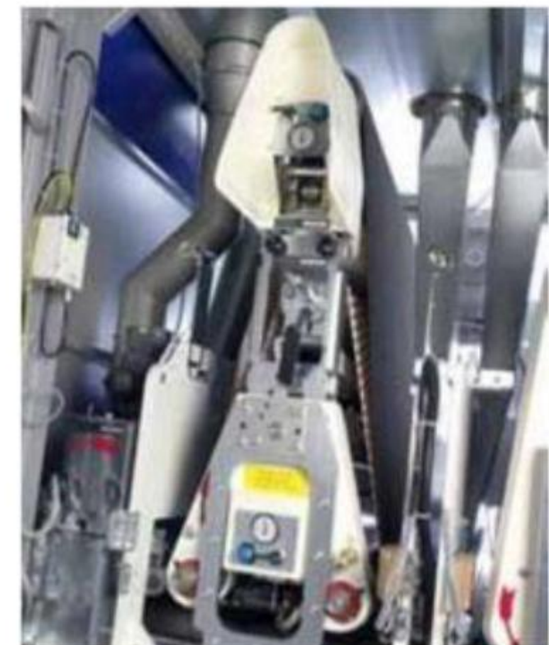
Longitudinal sanding unit (with pressure segment belt)
