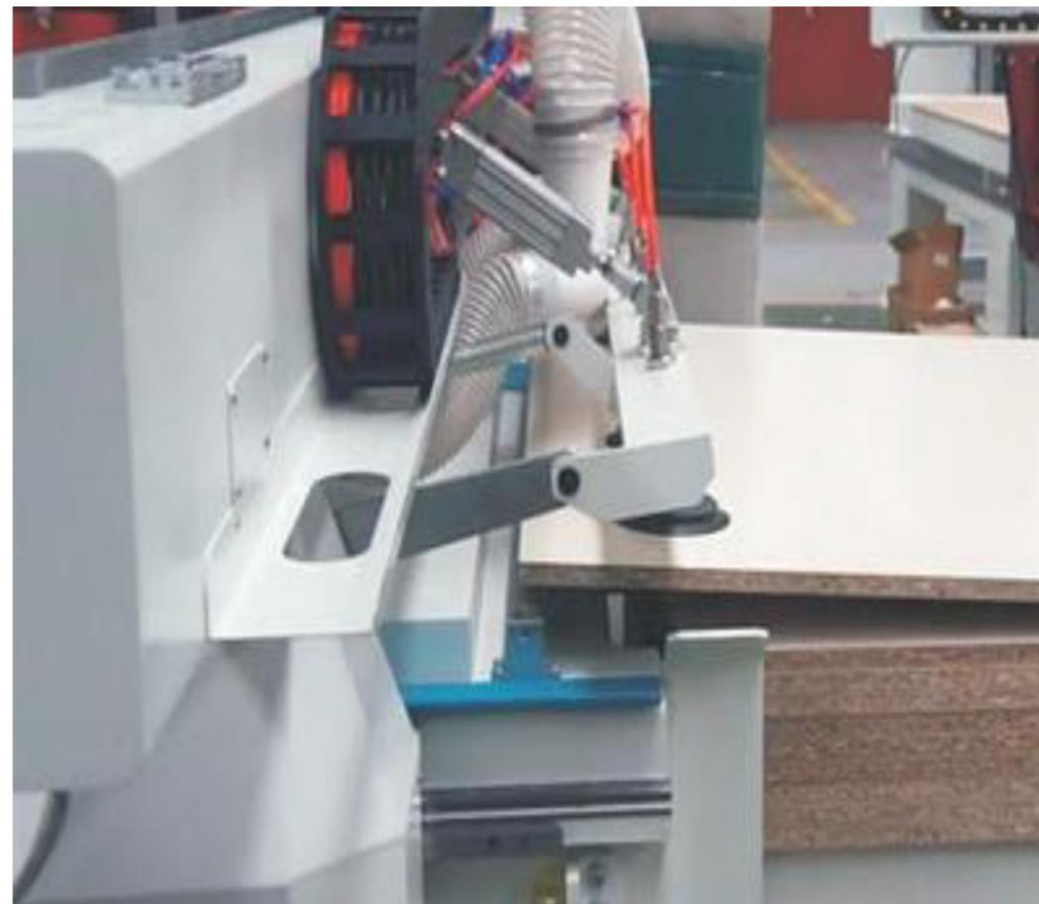
Automatic feeding of planks
